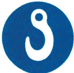
Figure 4: Decal on lifting eyes
