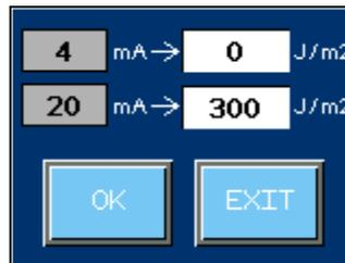
Associate the values 4 and 20 mA to the minimum and maximum Dose (Irradiance). Touching "OK", the user calibrates the 4/20 mA output.
