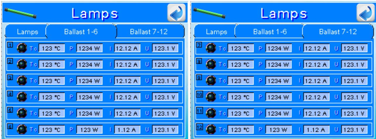
This screen displays the parameters of temperature, power, current and voltage of each lamp.
