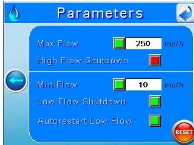
this screen allows to set alarm thresholds.
